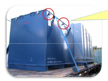
Can you see the problem with the lid closure clips? Could the tiedowns have caused this? Be careful with any shipping container that could be "opened" by the downward pressure from the tiedowns.
